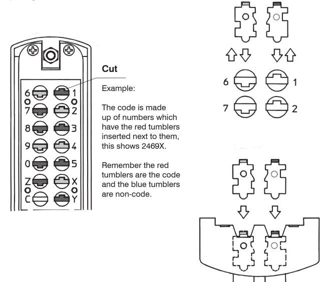
While holding knob in clear position make sure the blue or red colored end of the tumbler is facing upwards. Make sure notch is placed in the correct insert of the tumbler slot. See example.
